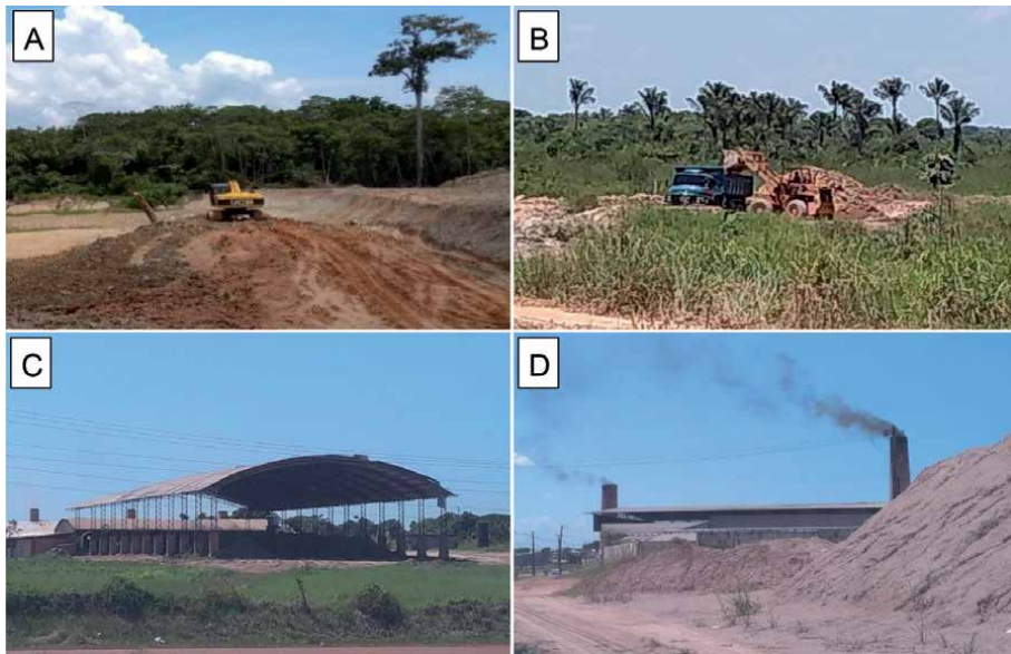
Figure 5. Processes of extraction (A), transport (B), and storage of clay raw material (C, D) in the study area. Source: The authors (2020).
